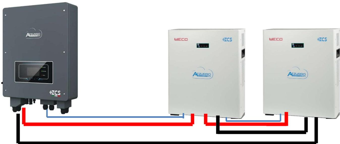
Figure 2 - example of connections with two batteries
