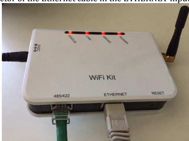
Figure 136 – Ethernet cable connected to the datalogger
