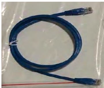
Figure 17 – Communication cable between WeCo 4k4 batteries
