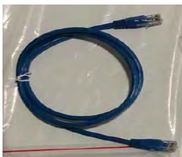
Figure 38 – Communication cable between WeCo 5K3XP batteries
