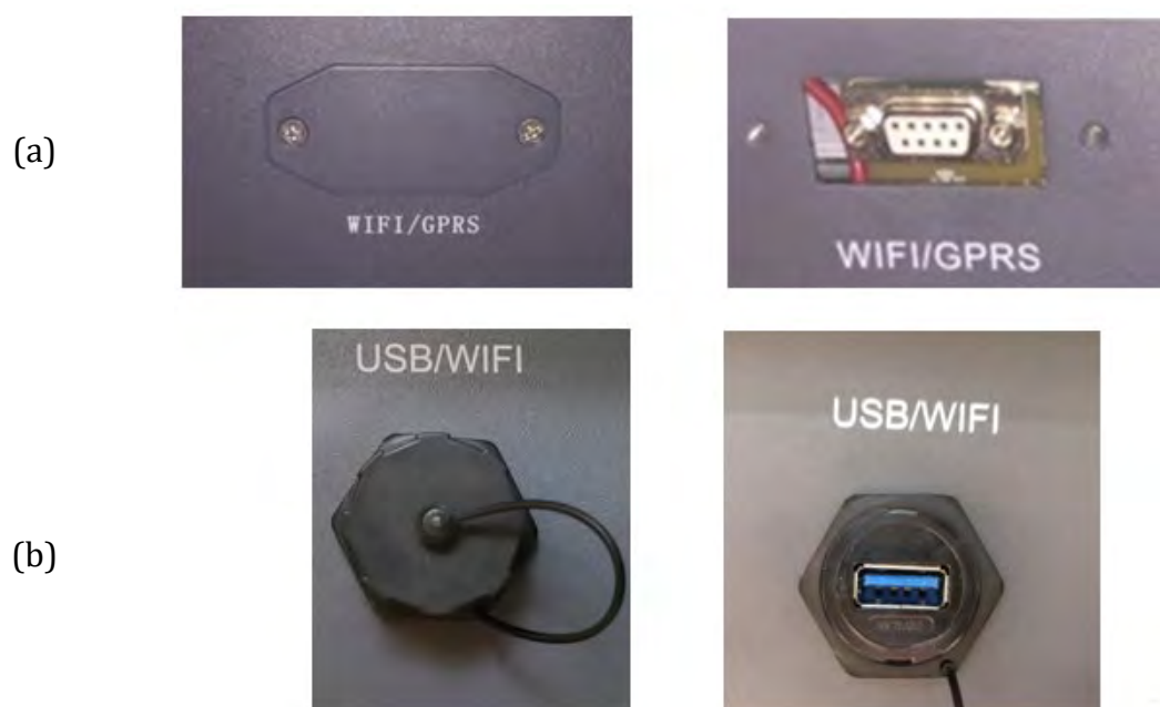
Figure 91 – Port for external Wi-Fi adapter
