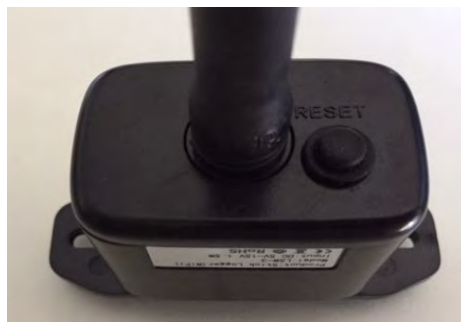
Figure 108 – Reset button on the Wi-Fi adapter
