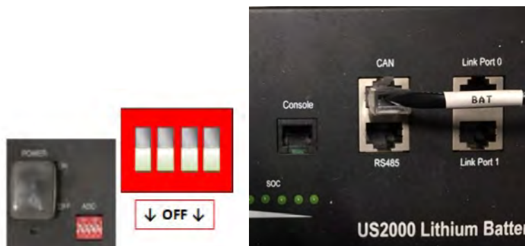
Figure 12 - Connecting the communication cable to the Pylontech battery
