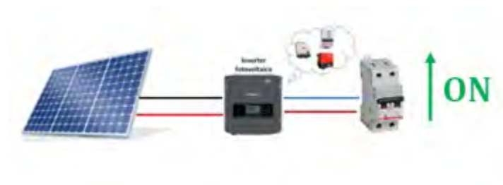
Figure 73 – Switching on the photovoltaic inverter
