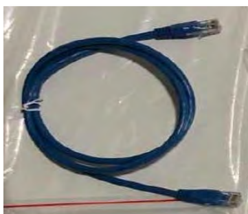
Figure 51 – Communication cable between AZZURRO 5000 batteries
