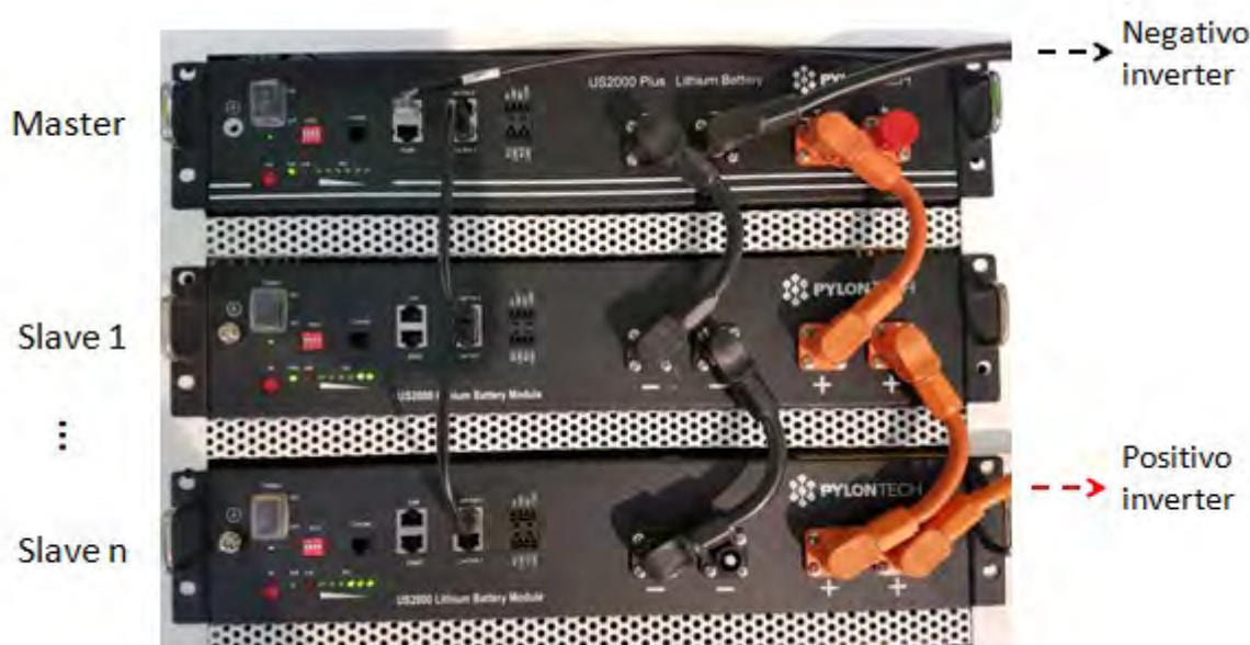
Figure 11 – Connecting three Pylontech batteries in parallel
