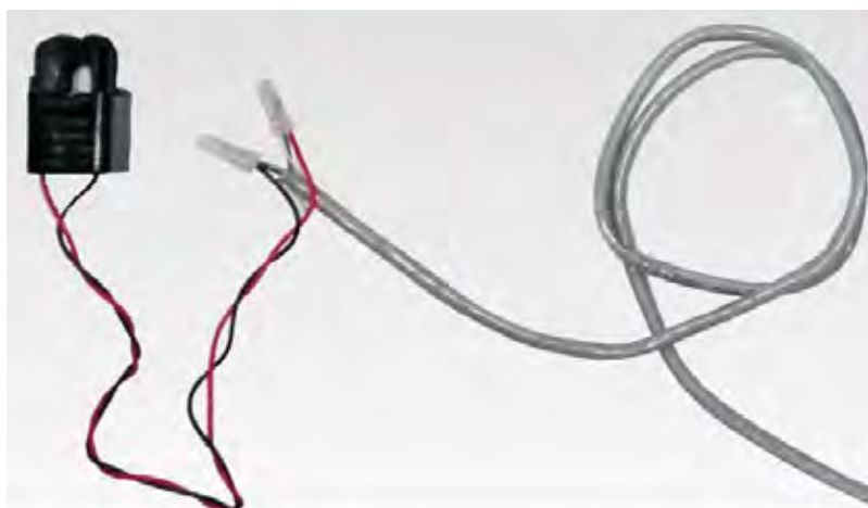
Figure 56 – Extending the cable of the CT current sensor
