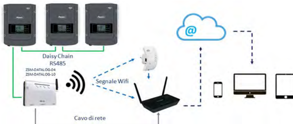
Figure 128 – Diagram for connecting the ZSM-DATALOG-04 / ZSM-DATALOG-10 datalogger
