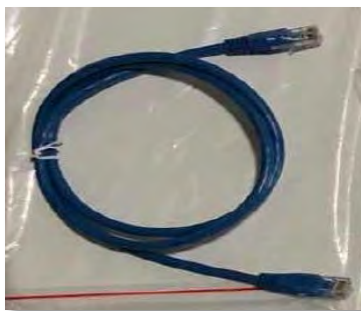
Figure 51 – Communication cable between AZZURRO 5000 batteries
