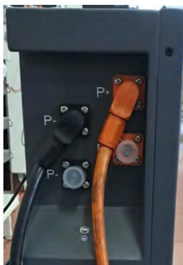
Figure 16 – Terminal block of the AZZURRO ZSX 5120 battery
