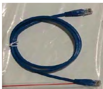
Figure 24 – Communication cable between WeCo 4k4 PRO batteries
