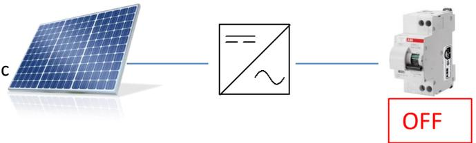
Make sure that there is a domestic load of at least 200 W. To make certain, use a current clamp to measure the current present on the phase under the import/export meter. The current will enter from the grid to the utility.
