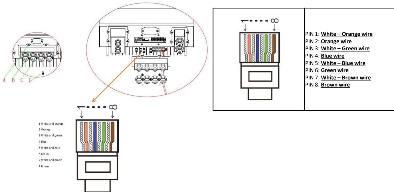
a) Logic interface for AS/NZS 4777.2:2015, also known as inverter demand response modes (DRMs). The inverter will detect and initiate a response to all supported demand response commands within 2s. The inverter will continue to respond while the mode remains asserted.
