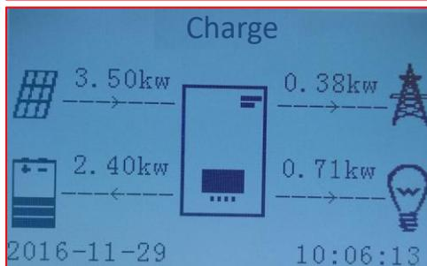
When the battery is fully charged, or when the charging power is limited (to preserve the integrity of the battery), the excess energy will be exported to the grid.
