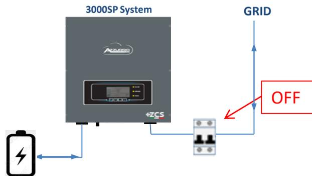
Make sure the PV system is not producing power on any phase where the PV system is connected, then open the AC circuit breaker dedicated to the PV inverter to verify that no power is being produced.
