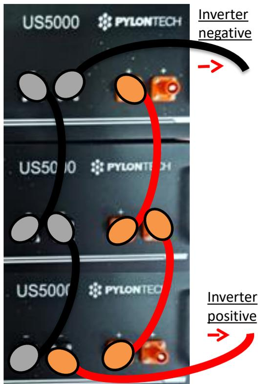
**Power connections between batteries and inverter:**
