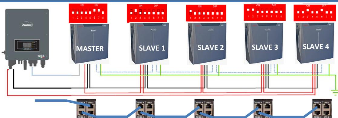
Set the battery channels in the inverter.
