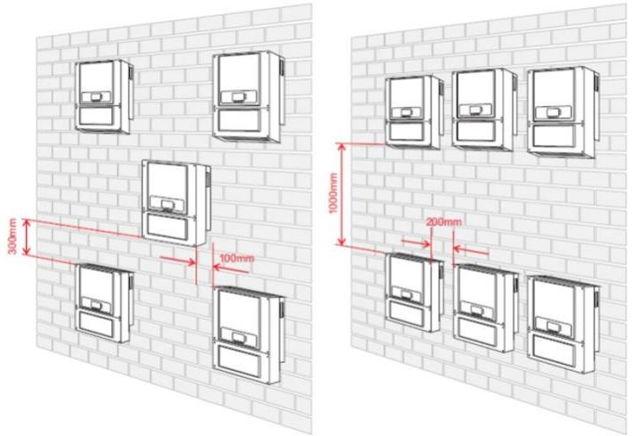
Correct installation in vertical position
