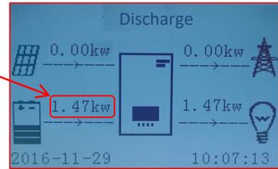
The photovoltaic system remains at zero.
