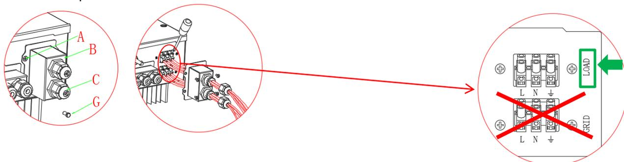
**1)** Unscrew the 4 screws (A) of the central cover with a screwdriver.
