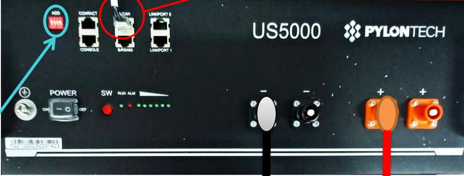
**Note:** DIP switches must be set as per the factory settings, all in the OFF position (00000)
