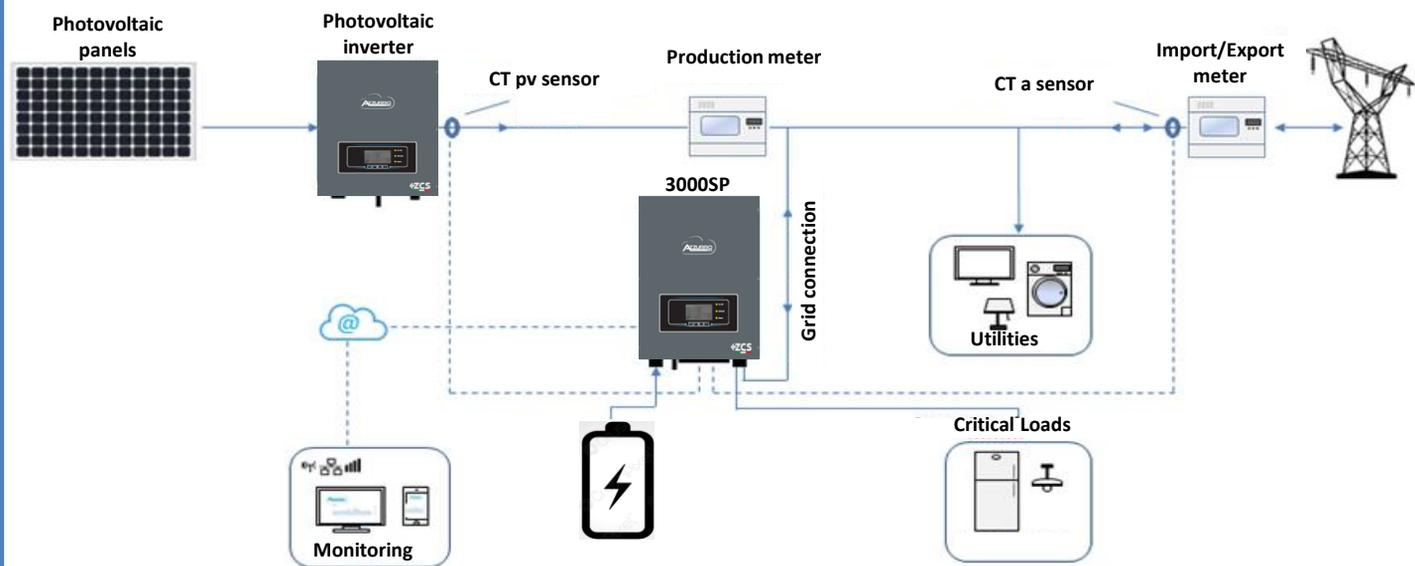
The wiring diagram for the 3000SP single-phase storage system is shown above.
