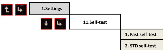
**Note:** the STD self-test is the same as the Fast self-test except that the waiting times are longer (about 45 minutes for the standard self-test compared to 12 minutes for the FAST self-test).
