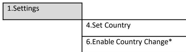
Select the code corresponding to the current legislation in the installation country (see table below) which can be set using the “Up” and “Down” keys, press “OK” to move to the next character and confirm.
