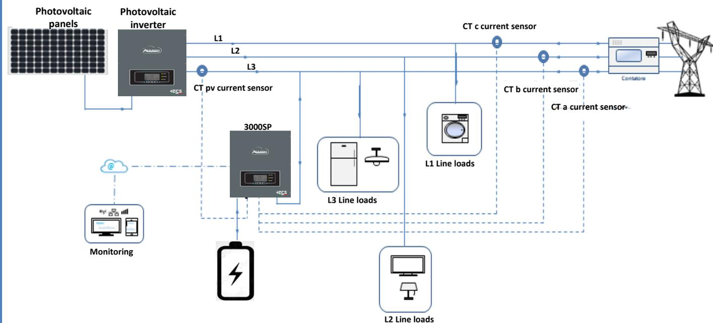
The wiring diagram for the 3000SP three-phase storage system is shown above.
