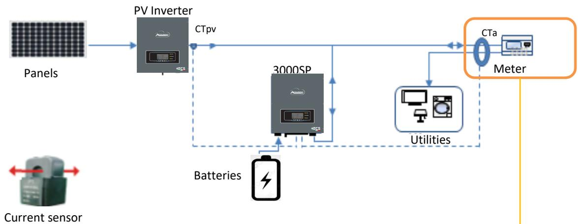
The sensor must include all phase cables entering or leaving the meter.
