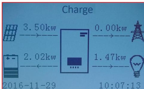
When the power produced from the photovoltaic system is greater than the energy required by the loads, the 3000SP system will charge the battery with the excess energy.
