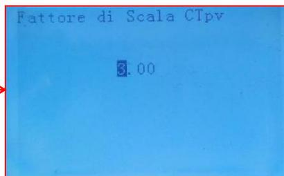
**NOTE:** The CTpv scale factor is the multiplying coefficient of the power value read by the CTpv sensor on the phase in which it is installed.
