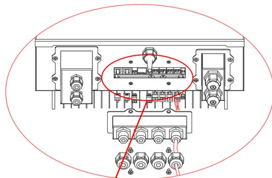
Replace the cover and secure it with the four screws; then tighten the cable glands.
