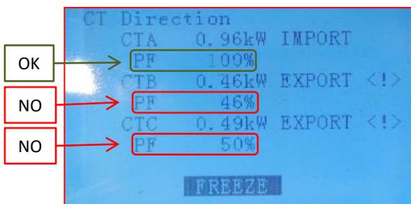
Block the CTs by pressing the arrow so that the word **FREEZE** appears at the bottom and then confirm with the fourth button
