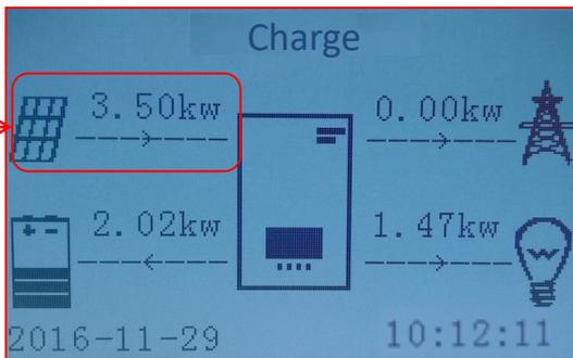
10) Compare the value of the photovoltaic power shown on the storage inverter's display with that indicated by the photovoltaic inverter, making sure that they are almost equal.
