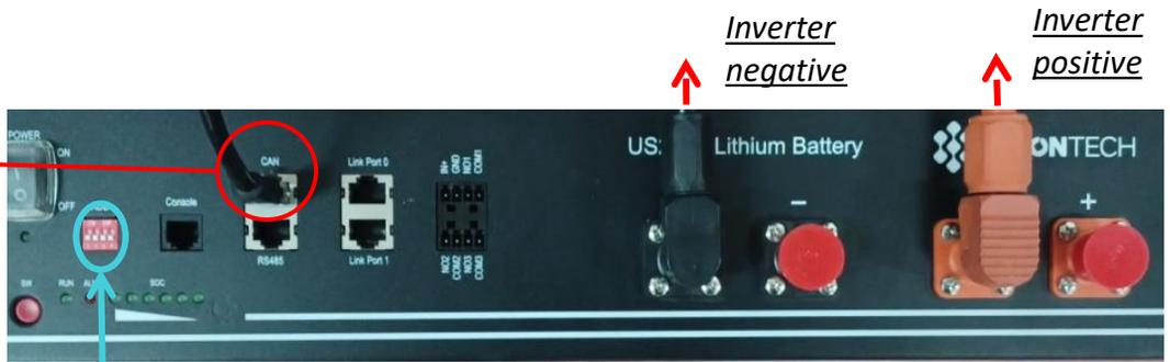
**Note:** DIP switches must be set as per the factory settings, all in the OFF position (00000)
