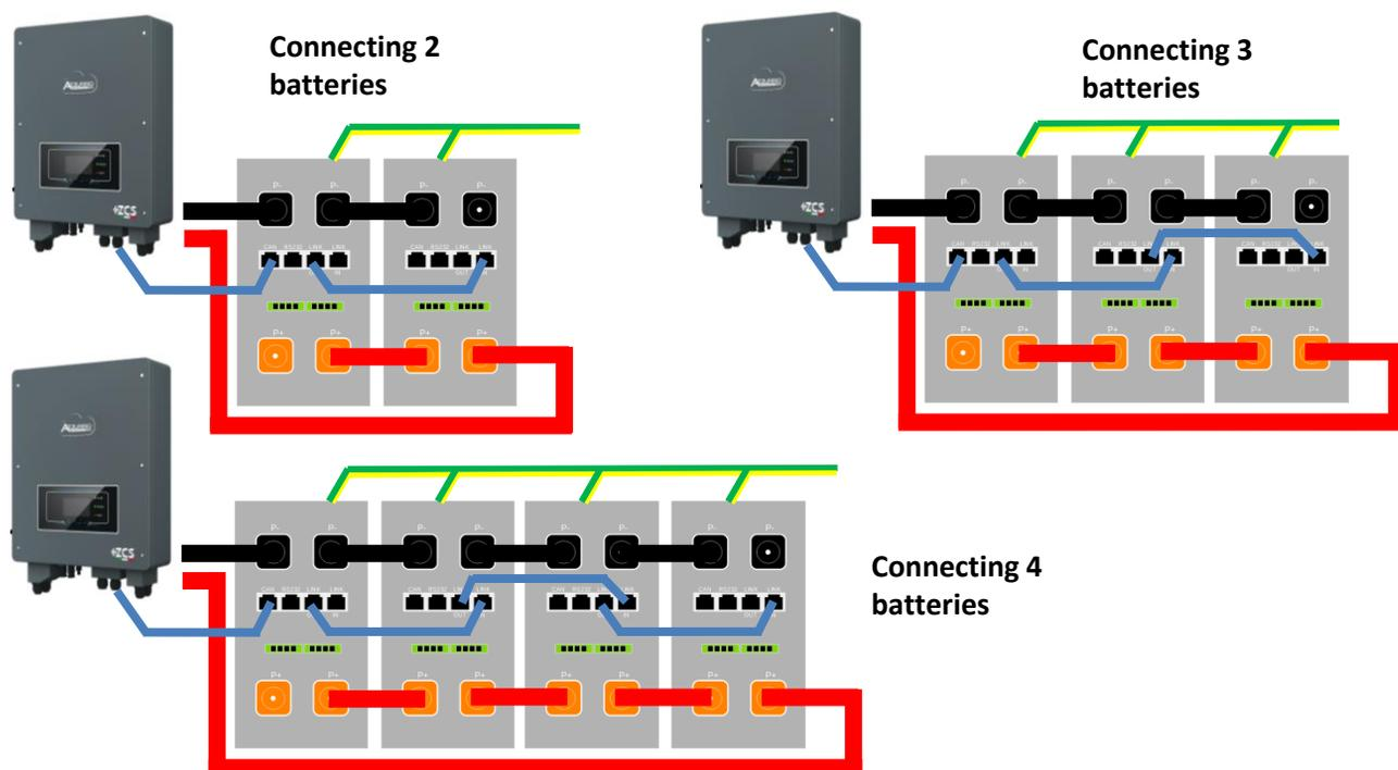
Set the battery channels in the inverter.
