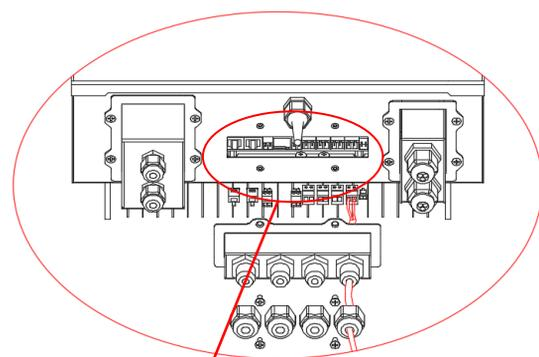
Correctly position the current sensors (CT):
