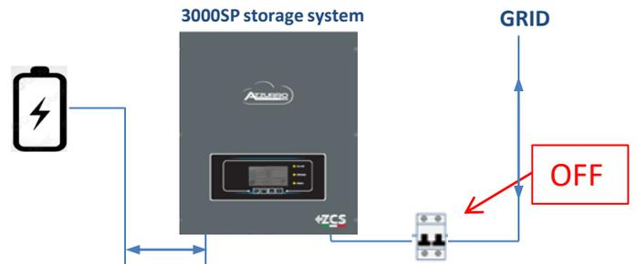
Make sure the PV system is not producing any power on the phase where the 3000SP system is connected, then open the AC circuit breaker dedicated to the photovoltaic inverter to verify that no power is being produced.
