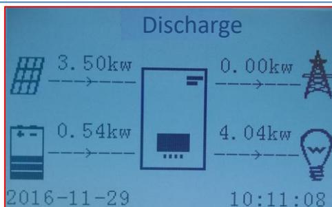
When the power of the photovoltaic system is once again less than the power required by the loads, the system will use the energy stored in the battery to power the domestic utilities.
