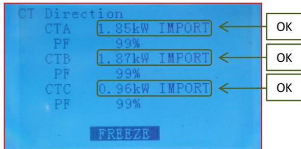
If each sensor has been correctly positioned on its reference phase, the **PF** value (phase shift between voltage and current) will be greater than 90% on all three phases.
