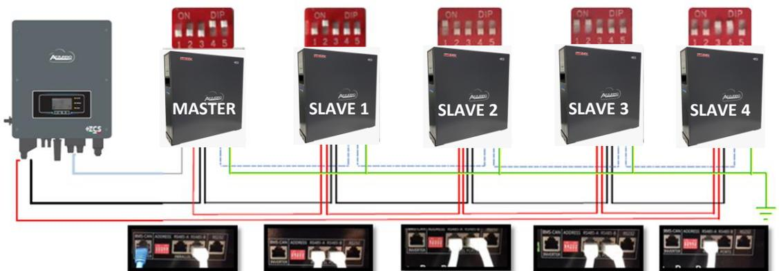
Set the battery channels in the inverter.
