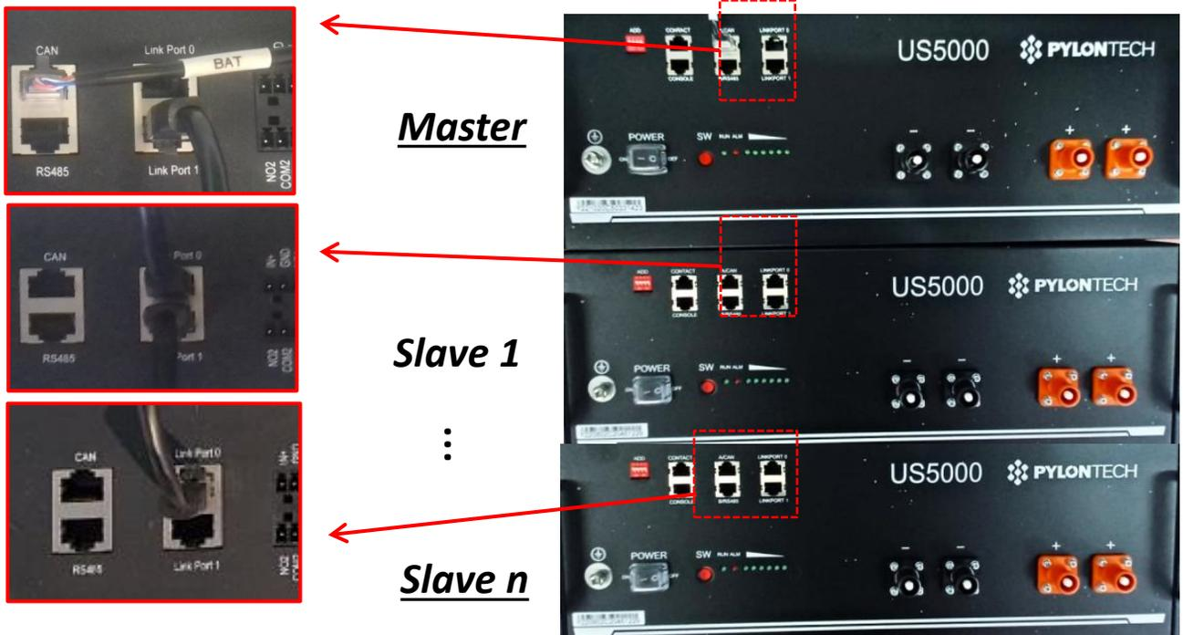
**Communication connections between batteries and inverter:**
