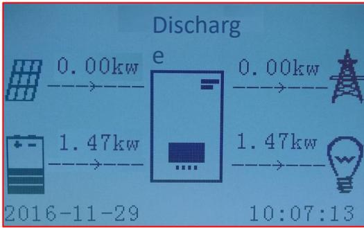
7) Once the countdown is over, the batteries will start to deliver power according to the availability towards the utility, trying to reset the consumption from the grid.
