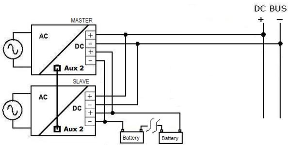
Power supply can be paralleled to increase the output power, devices can be paralleled for 1+1=2 to obtain the double power of a single unit. Only SIZE 3 devices can be connected in parallel to attain the sum of the current at the same output voltage. It is necessary to use a standard UTP or order Cable code: RJCONN45 for RJ45, and connect to Aux2 of each device. The communication protocol is based on CAN2.0A standard.
