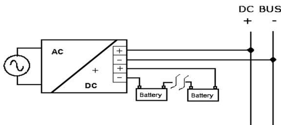
Typical application for All In One device, one output for Load "DC Bus", one Input / Output for connection to the battery.
