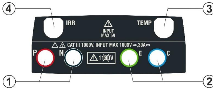
Fig. 2: Description of the upper part of the instrument
